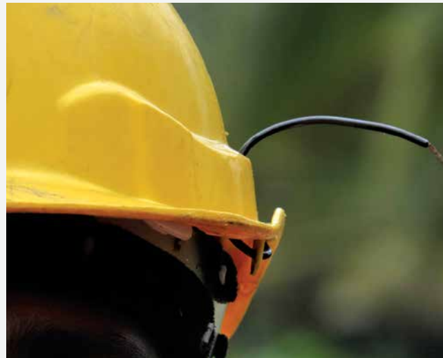
Helmet mounted induction tester
