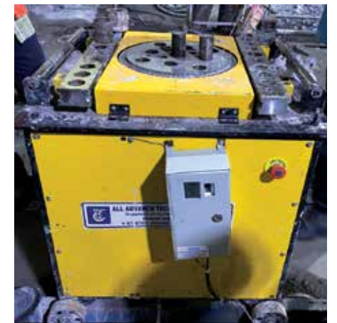
Bar bending machine equipped with fingerprint authentication
